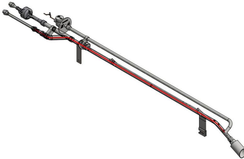
Figure 3: Highlight of fiber optic layout in flare pilot
